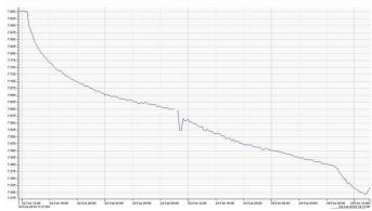
The graph shows the dramatic 80cm drop in flood water levels achieved in two days in February 2014 by fully opening the sluice at Monk's Leaze Clyse at the head of the Sowy (pictured right, branching off from the Parrett).
